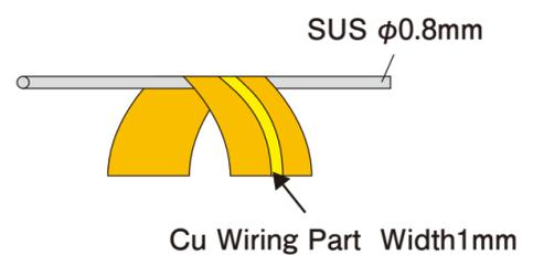
From this result, we observed the crack formation on the test specimen having thicker Ni plating film of the conventional type film. On the other hand, we could not observe any crack formation on the FPF and SOF films, and we found that they could gain good bending resistance.
