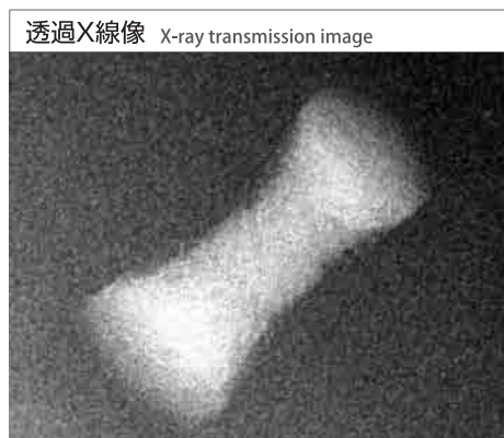
穴径 80μm 板厚 200μm めっき膜厚 15μm Hole diameter 80 μm Board thickness 200 μm Film thickness 15 μm
